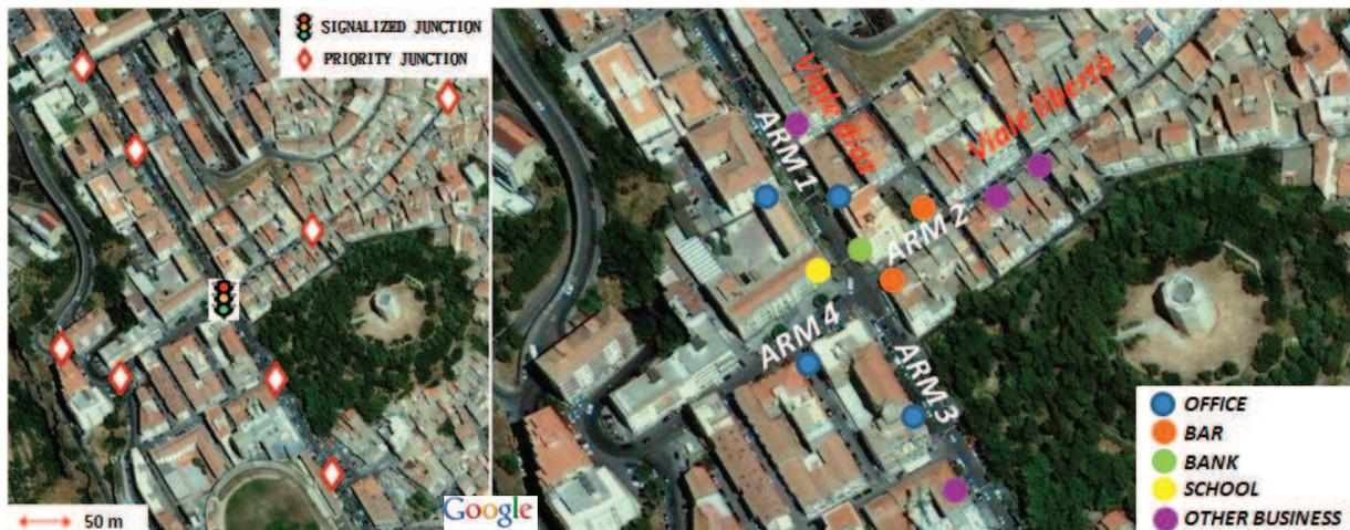
Figure 1. Type of junctions (left) and layout of the signalised intersection studied in Enna, with characterisation of business activities (right)
