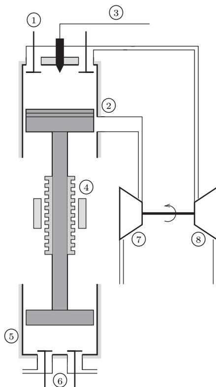
Fig. 1 Free-piston engine [22]
