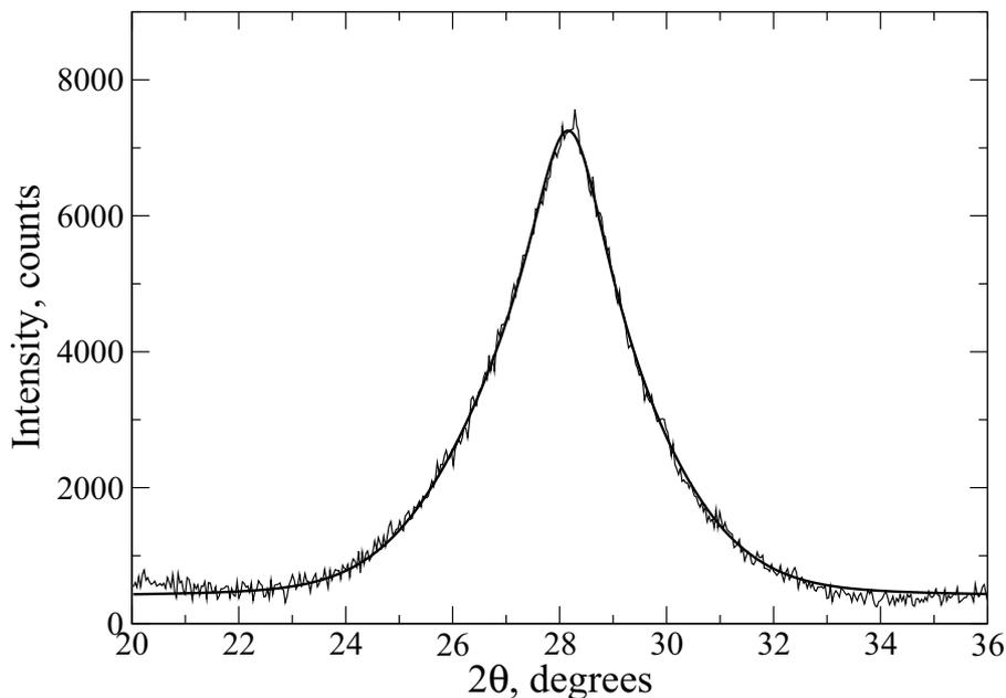
Figure 6: Pseudo-Voigt fit to the (111) peak of the XRD pattern for C<sub>11</sub>-NCs after subtraction of a linear baseline.
