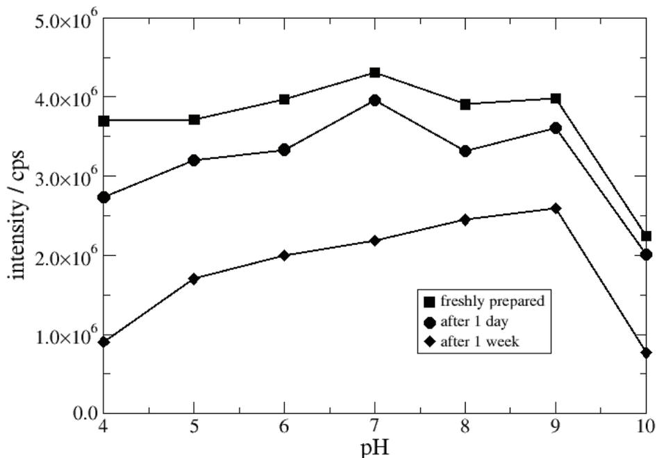
Figure 5: Luminescence intensity ( $\lambda_{max}$  is given in figure 6) of alkylated silicon quantum dots in 1% v/v THF/water at different times after preparation of the sols (excitation wavelength = 330 nm). The samples were stored in glass vials in the dark under ambient conditions and no attempt was made to purge the suspensions of oxygen.
