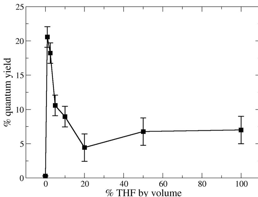
Figure 2: Luminescence quantum yield of alkylated silicon quantum dots against % THF by volume in THF/water mixtures. The amount of silicon quantum dots is the same in each sample. The excitation wavelength was 330 nm and the intensity given is that at the peak of the PL spectrum at 665 nm.
