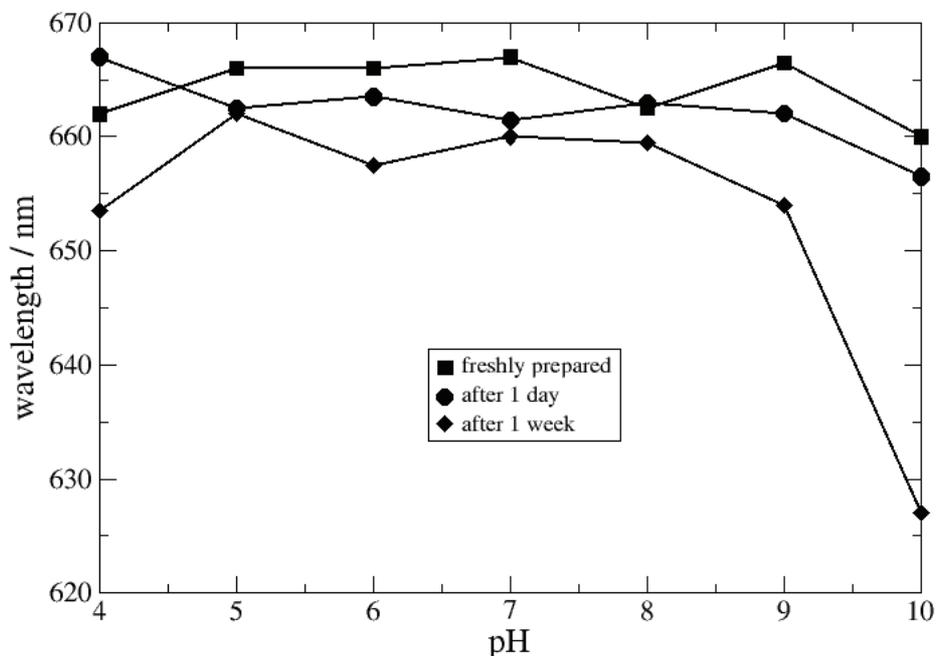
Figure 6: Wavelength of the orange peak in the luminescence spectra of alkylated silicon quantum dots in 1% v/v THF/water at different times after preparation of the sols (excitation wavelength = 330 nm). The samples were stored in glass vials in the dark under ambient conditions and no attempt was made to purge the suspensions of oxygen.
