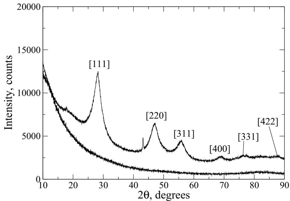
Figure 5: XRD pattern of a film of  $C_{11}$ -NCs cast from dichloromethane solution. The peaks are assigned to the indicated lattice planes of crystalline silicon. The lower curve is the background scattering from the blank.
