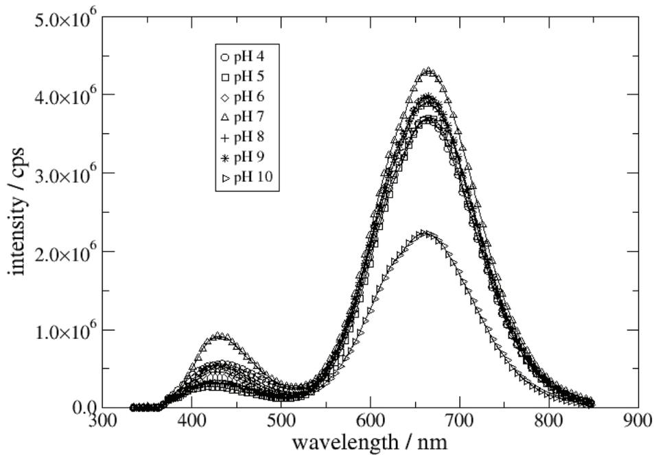
Figure 4: Luminescence spectra in buffers of different pH for alkylated silicon quantum dots in 1% v/v THF/water. The excitation wavelength was 330 nm.
