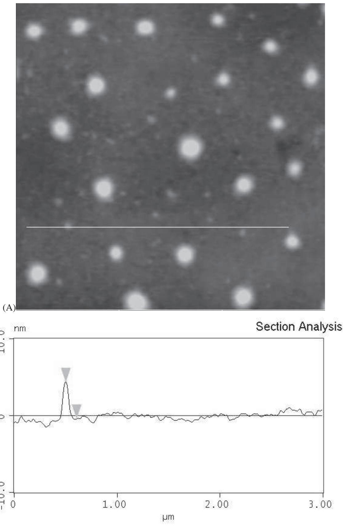
Figure 8: (A) Tapping mode AFM image of alkyl-SiNCs deposited from the vapor onto undecyl-capped Si(111) surfaces. The grayscale corresponds to 20 nm and the image area is  $3 \times 3 \mu\text{m}$ . (B) zoom and line section of an island one particle high.
