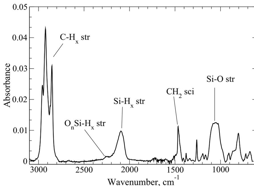
Figure 2: FTIR spectrum in normal transmission of C<sub>11</sub>-SiNCs deposited from dichloromethane solution on a 1 cm<sup>2</sup> Si(100) chip. The background was the same chip before deposition of the alkyl-SiNCs.
