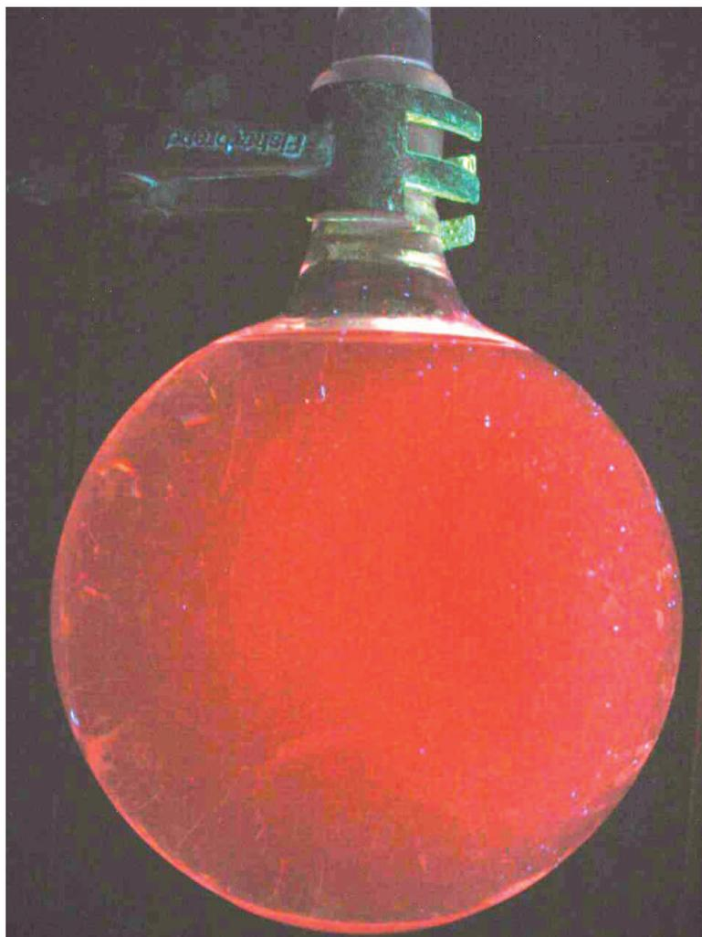
Figure 1: A 1L flask containing 0.01% v/v THF/water in which alkylated silicon quantum dots have been dispersed. The orange luminescence from the silicon was excited by a hand-held UV lamp ( $\lambda = 365$  nm). The contrast and brightness of the photograph has been enhanced for printing, but the image has not otherwise been processed.
