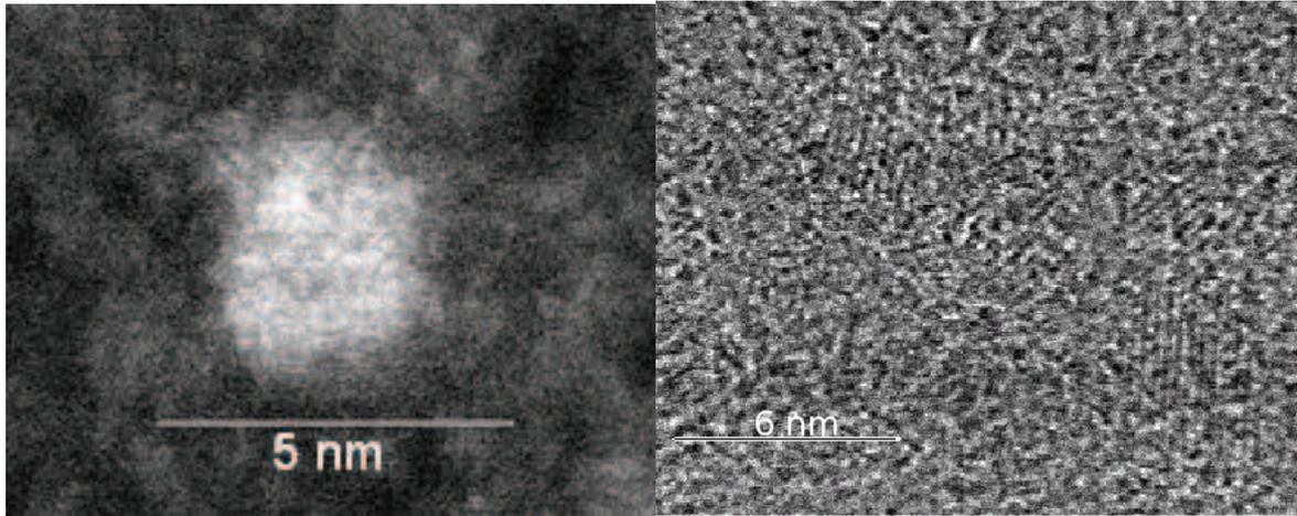
Figure 7: Left: STEM HAADF (aberration-corrected) images of a single  $C_{11}$ -SiNC particle; the white region corresponds to the Si core. Right: bright field image showing several particles in which the lattice fringes due to [001] planes are visible. In both cases, the beam energy was 100 keV and the resolution was about 0.1 nm.
