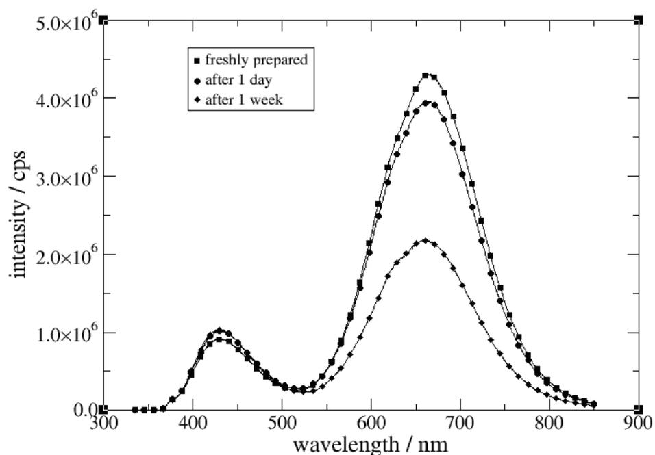
Figure 7: Ageing effect on luminescence spectra in pH 7 buffer for alkylated silicon quantum dots in 1% v/v THF/water (excitation wavelength = 330 nm). The samples were stored in glass vials in the dark under ambient conditions and no attempt was made to purge the suspensions of oxygen.
