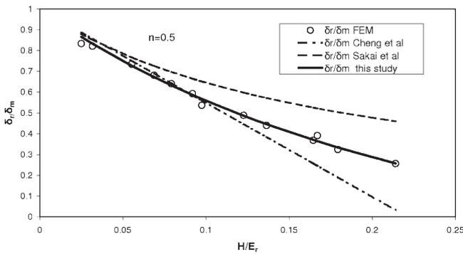
FIG. 3. Comparison of the relationship between the ratio of residual depth to maximum depth and the ratio of hardness to contact modulus for materials with severe work hardening ( $n = 0.5$ ) determined by different workers and finite element simulation.
