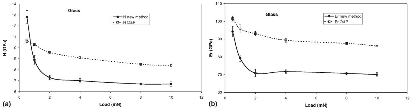
FIG. 13. Comparison of (a) hardness and (b) reduced modulus for soda lime glass using O & P and the new model suggested here [i.e., Eq. (28)].
