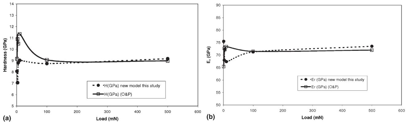
FIG. 11. Comparison of (a) hardness and (b) reduced modulus of fused silica using the Oliver and Pharr method (O & P) and the new model suggested here [i.e., Eq. (28)].
