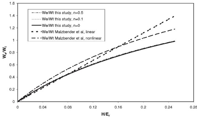
FIG. 9. Comparison of the variation of  $W_e/W_t$  with  $H/E_r$  determined in this study [i.e., Eq. (23)] and the linear and nonlinear expressions given by Malzbender et al.<sup>6,18</sup> [i.e., Eqs. (14) and (24)].
