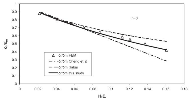
FIG. 1. Comparison of the relationship between the ratio of residual depth to maximum depth and the ratio of hardness to contact modulus for elastic-perfectly plastic materials ( $n = 0$ ) determined by different workers and finite element simulation.
