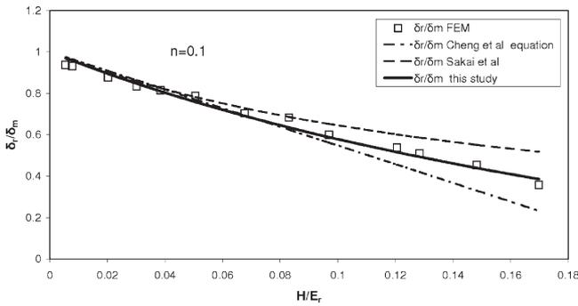
FIG. 2. Comparison of the relationship between the ratio of residual depth to maximum depth and the ratio of hardness to contact modulus for materials with work hardening ( $n = 0.1$ ) determined by different workers and finite element simulation.
