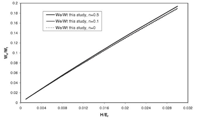
FIG. 10. Localized plot of  $W_e/W_t$  versus  $H/E_r$  for soft materials (with low  $H/E_r$ ) with different levels of work hardening. The effect of work hardening is negligible.
