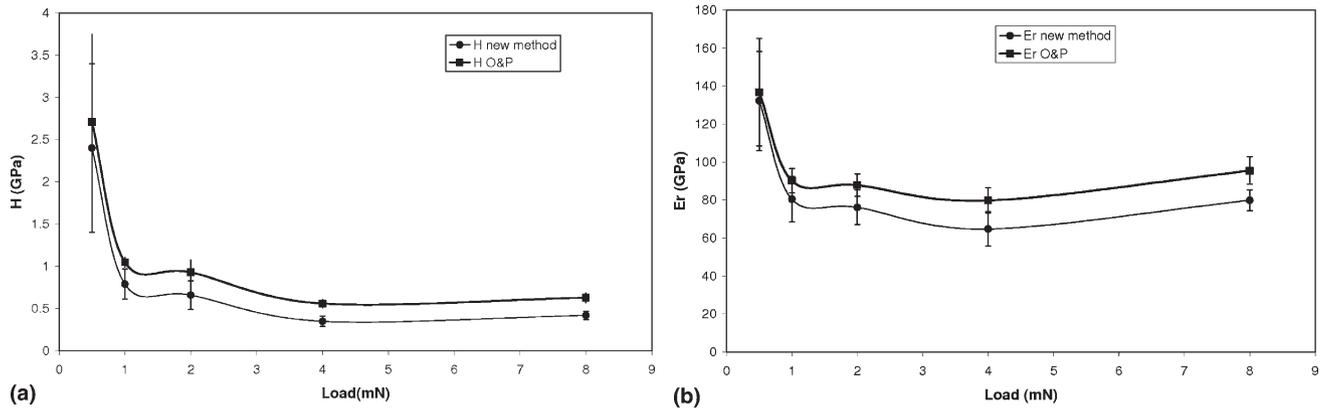
FIG. 12. Comparison of (a) hardness and (b) reduced modulus of aluminum using O & P and the new model suggested here [i.e., Eq. (28)].
