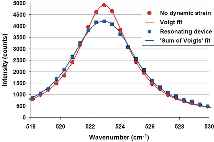
Figure 8: The Raman profile of silicon appears broadened during resonance.
