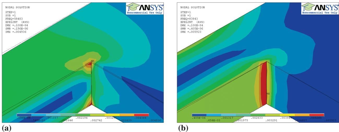
Figure 9: Modelled strain intensity maps of a test structure showing (a) first out of plane and (b) first in plane mode of vibration for a free end amplitude of 10 $\mu$ m.
