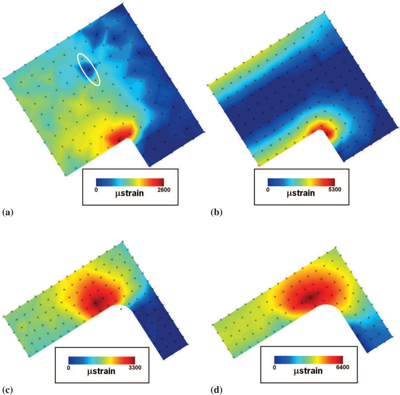
Figure 10: Strain induced during oscillation in (a) the first out of plane and (b) first in plane modes of vibration. Crosses indicate measurement points every 2  $\mu\text{m}$ . For each mode, corresponding high spatial resolution maps (points every 500nm) are shown in (c) and (d) respectively.
