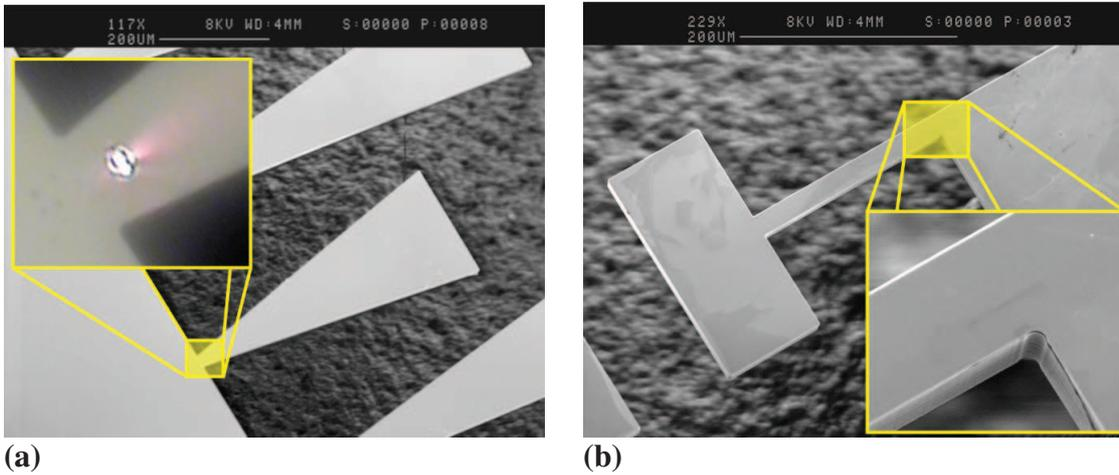
Figure 1: SEM images of the fabricated cantilever type test structures. The laser position for the experimental results in section 4 is highlighted in (a). The region mapped in section 5 is highlighted in (b).
