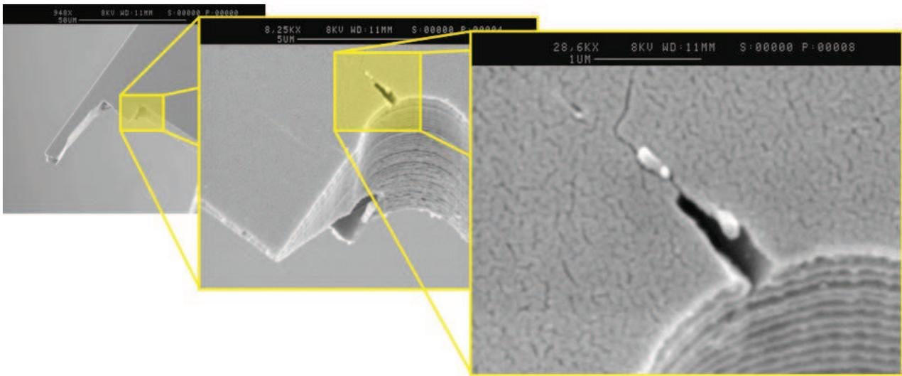
Figure 11: SEM images of the fractured device due to excessive in plane vibration.
