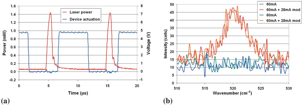
Figure 4: (a) A measurement of laser intensity shows an on:off ratio of 23:1. (b) Comparison of Raman profile obtained from 1/16<sup>th</sup> and 0 duty cycles.
