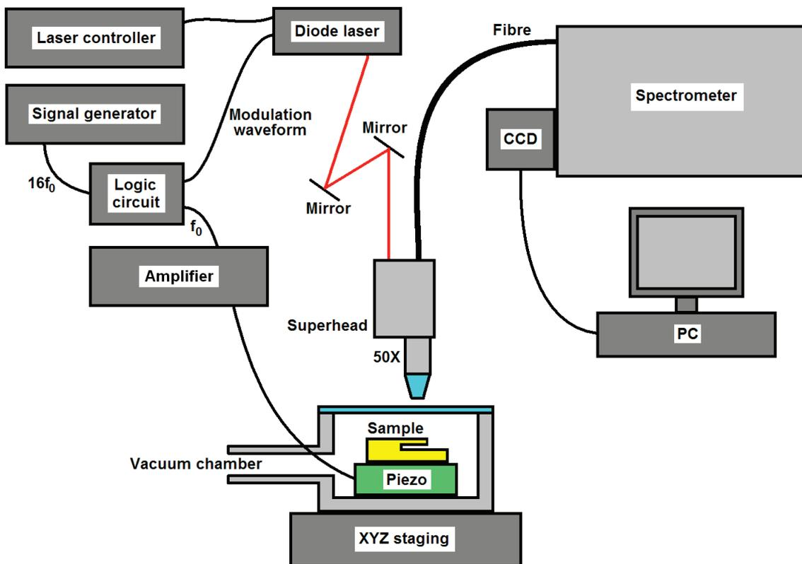
Figure 3: Schematic of the experimental setup for the strobed Raman measurements.
