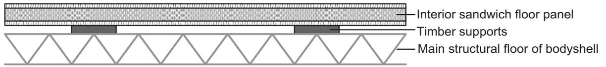
**Fig. 3.** A cross-section of the assumed configuration of the sandwich flooring.
