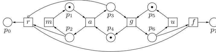
**Fig. 4.** An ENIM-system modelling a producer/consumer system with the actions: ‘make item’  $m$ , ‘add item to buffer’  $a$ , ‘get item from buffer’  $g$ , ‘use item’  $u$ , ‘producer retires’  $r$ , and ‘consumer finishes’  $f$ . Note: the producer can only retire if the buffer is empty (i.e.,  $p_3$  is empty).
