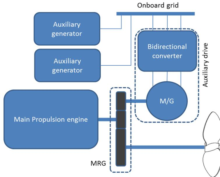
Fig. 1: Auxiliary drive topology.
