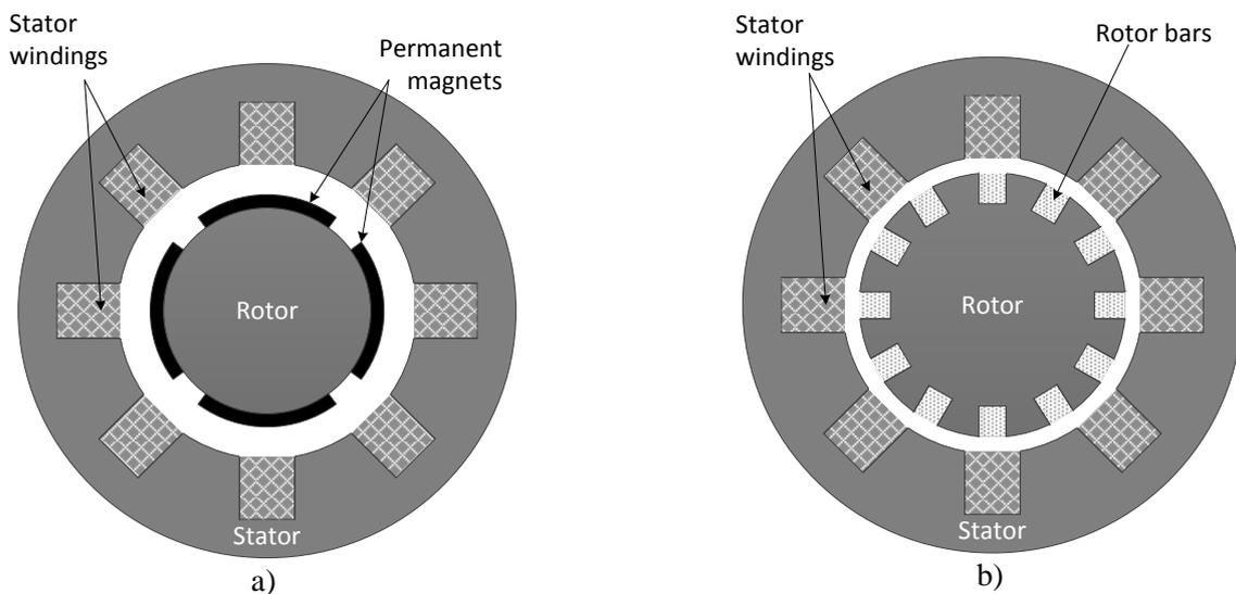
Fig. 2: Cross-sectional comparison of a) Permanent magnet and b) Induction machines.
