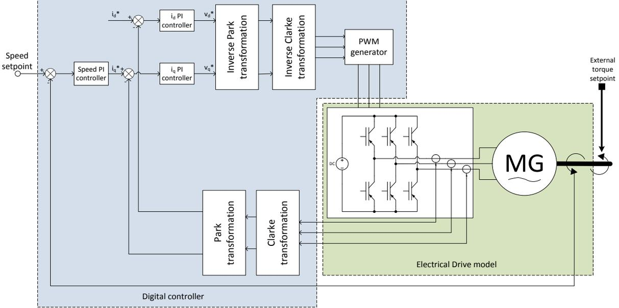
Fig. 5: Auxiliary drive model overview.
