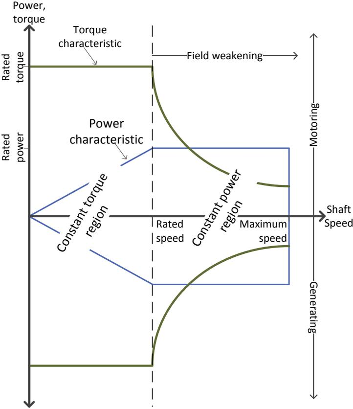
Fig. 3: Electrical machine operating envelopes.
