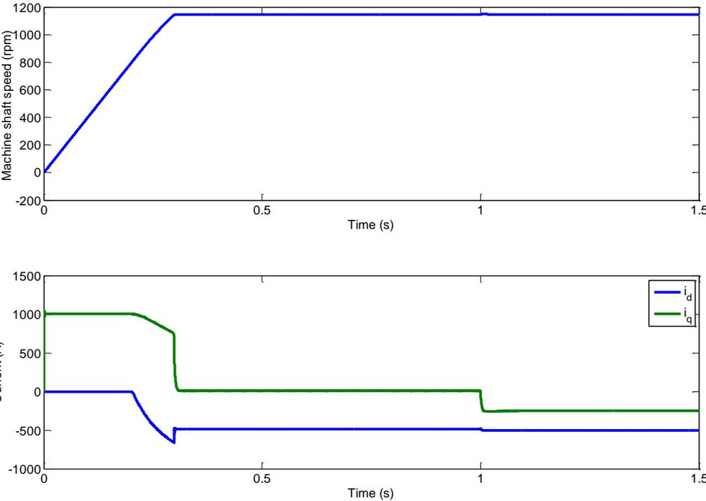
Fig. 8: Step response of PMSM drive in generating mode.
