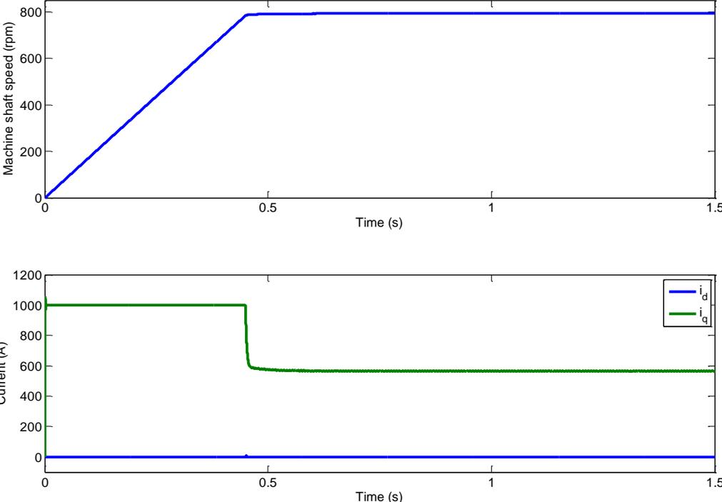
Fig. 7: Step response of PMSM drive when motoring.
