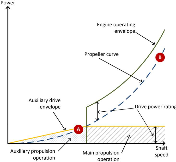
Fig. 4: Operating envelopes of auxiliary drive, main engine and propeller curve. Operating point A corresponds to low speed propulsion, while operating point B is sailing at rated speed.
