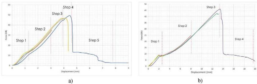
Fig. 4. Force-displacement graph for CF punch tip; a) SPR1.2; b) SPR4.1.
