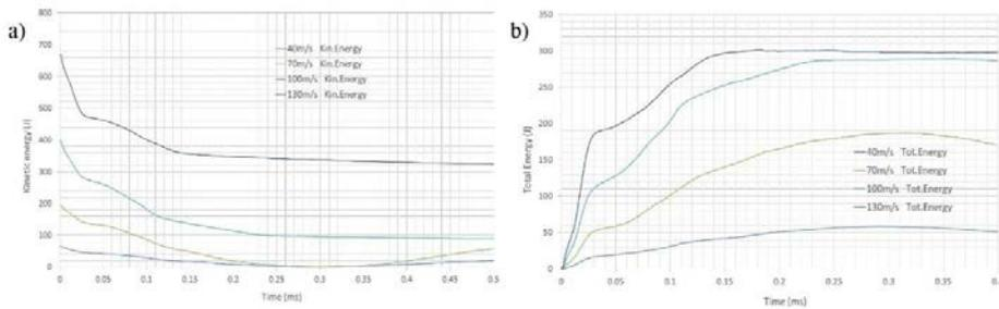
Fig. 7. HVI results for GFRP laminates; a) Kinetic energy change of projectile; b) Total energy change of laminate.
