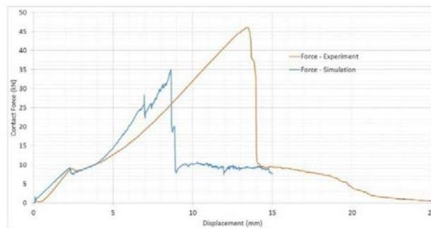
Fig. 6. Force-displacement graph for experiment and simulation (SPR4.1).
