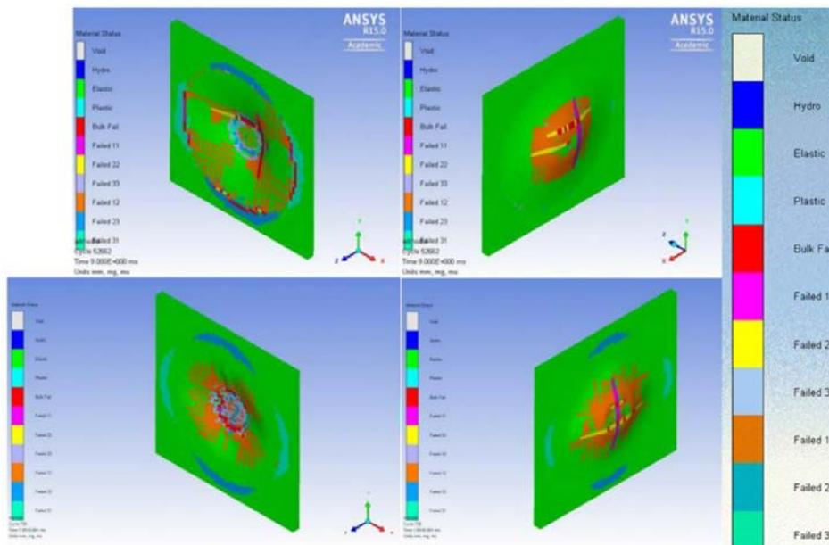
Fig. 8. QSP and HVI front and back face failure map comparison - top row QSP, bottom row HVI.
