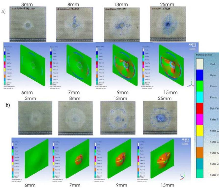
Fig. 5. Damage progression of laminates for SPR 4.1 with CF punch tip: a) impact face progression – experiment and simulation; b) back face progression – experiment and simulation.
