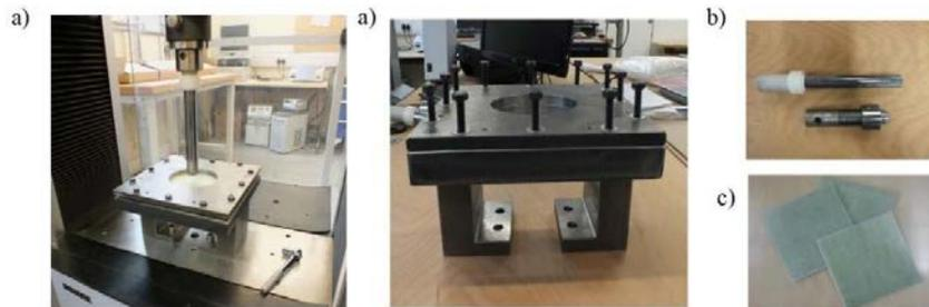
Fig. 1. Fixture and specimens used in the experiments; a) steel fixture; b) punch tips; c) GFRP samples.
