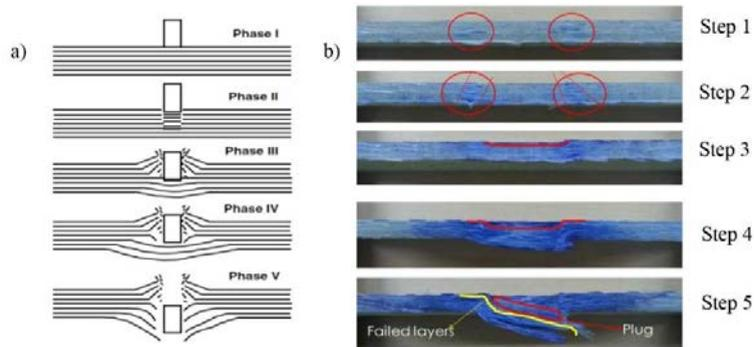
Fig. 3. Damage pattern of a) HVI; and b) QSP.
