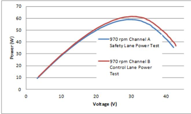
Figure 11: Power from the DC bus for diametrically opposite power lanes
