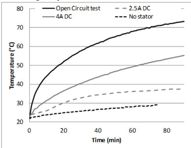
Figure 12: Base plate temperature variation with time for 100% speed open circuit test and static DC test for reference
