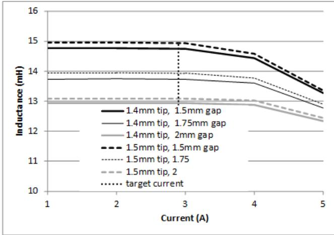
Figure 7: Finite element analysis predictions of inductance variation with current for alternative tooth tip configurations
