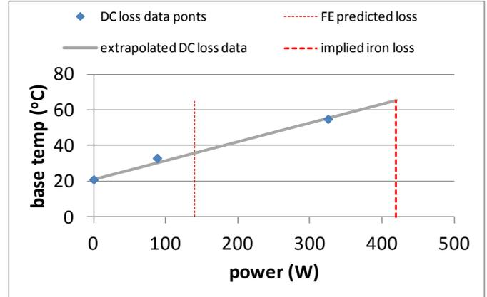
Figure 13: Relating base temperature rise of 90 mins to power loss
