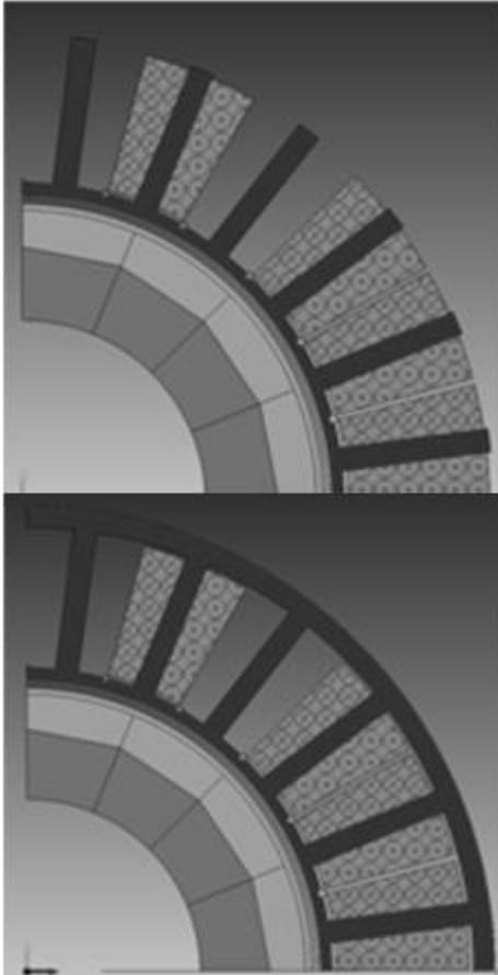
Figure 4: Fully closed slot design. Before (upper) and after (lower) back iron slotted over machine
