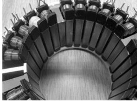
Figure 8: Final stator during assembly, prior to inserting in machine casing
