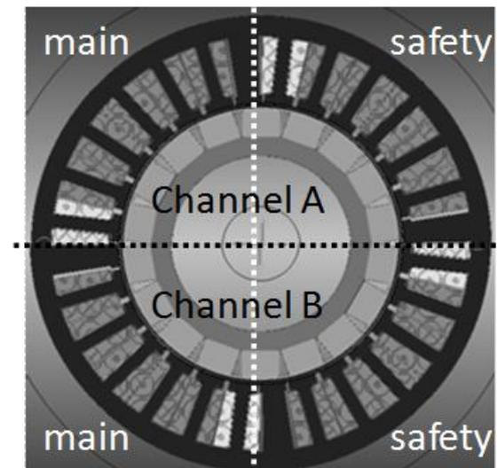
Figure 6: Coil layout of entire machine
