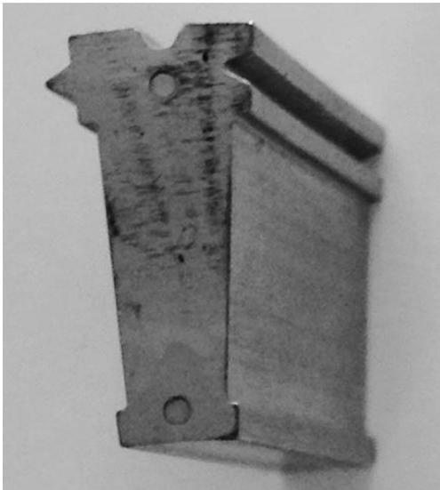
Figure 5: Single segmented stator tooth
