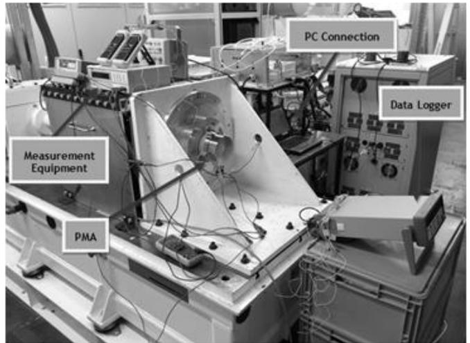
Figure 9: Machine mounted on test-bed
