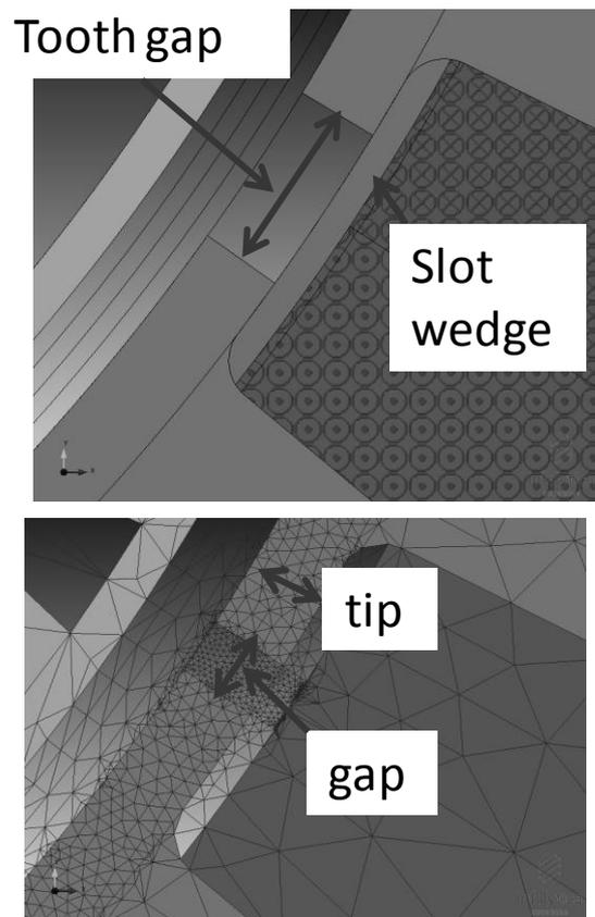
Figure 3: Slot wedge (upper) versus re-shaped tooth (lower) for equivalent magnetic performance
