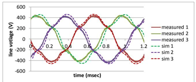
Figure 10: 50% Speed open circuit back emf results
