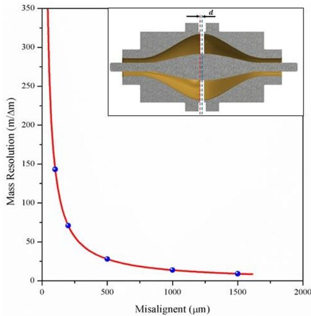
Figure 4: External electrode axial misalignment simulated mass resolution results with CAD model of exaggerated misalignment inset
