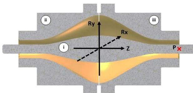
Figure 2: Ion trap axes, where i) is the internal “spindle” electrode, and ii) & iii) are the external electrodes
