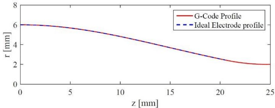
Figure 5: Overlay of ideal internal electrode profile with G-code approximation
