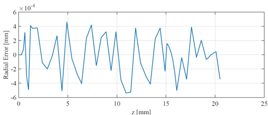
Figure 6: Resulting radial error when G-code profile is subtracted from ideal internal electrode profile
