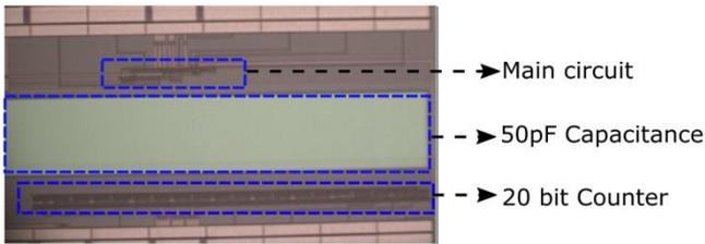
**Figure 7. Snapshot of the chip**
