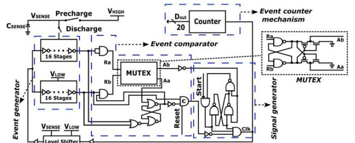
Figure 3. Asynchronous Implementation.
