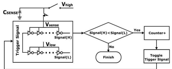
Figure 1. Iterative delay chain discharge method
