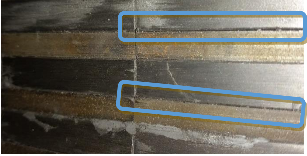
Fig. 8. Air-gaps Between Epoxy Retained Magnets and Pole Pieces
