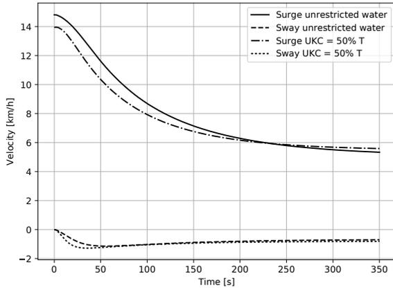
Figure 2: Surge and sway velocities during turning circle manoeuvre in unrestricted water and with an Under Keel Clearance of 50% Draught.
