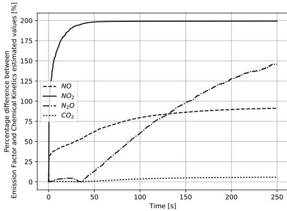
Figure 8: % difference in  $NO_X$  emissions between simulated and emission factor prediction with time during turning circle manoeuvre in confined water.
