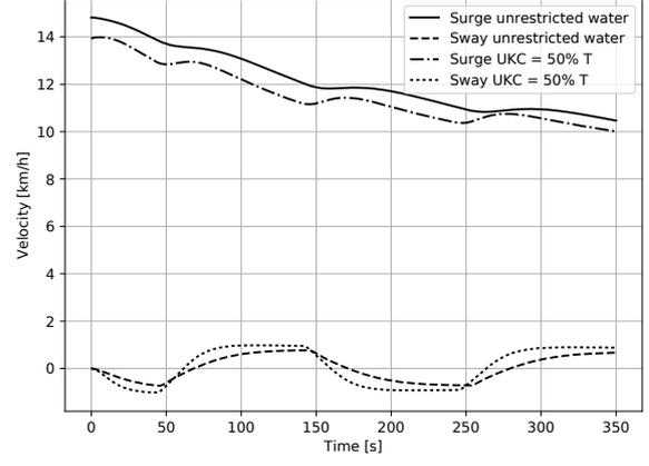
Figure 4: Surge and sway velocities during zig-zag manoeuvre in unrestricted water and with an Under Keel Clearance of 50% Draught.
