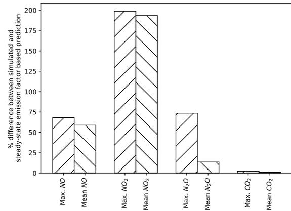
Figure 11: % difference in emissions between simulated and emission factor prediction during zig-zag in confined water.
