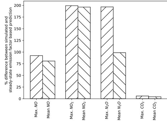
Figure 10: % difference in emissions between simulated and emission factor prediction during turning circle in confined water.
