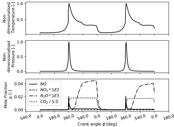
Figure 7: Effects of cylinder operating conditions on  $NO$  and  $CO_2$  formation as estimated from simulation.
