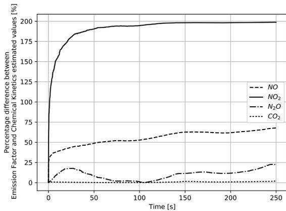
Figure 9: % difference in  $NO_X$  emissions between simulated and emission factor prediction with time during 20/20 zig-zag manoeuvre in confined water.
