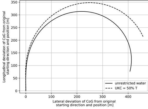
Figure 1: Ship track during turning circle in unrestricted water and with an Under Keel Clearance of 50% Draught.
