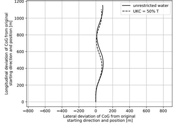
Figure 3: Ship track during zig-zag manoeuvre in unrestricted water and with an Under Keel Clearance of 50% Draught.
