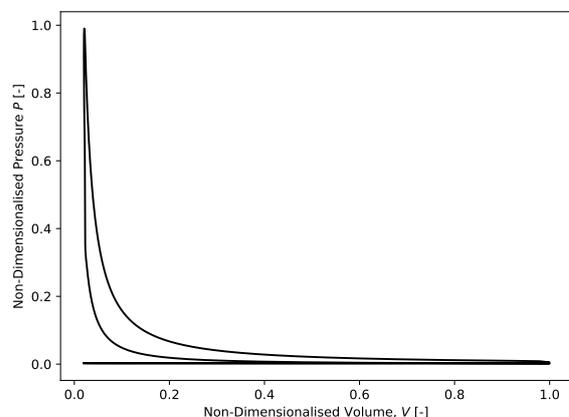
Figure 6: Indicator diagram from engine model.
