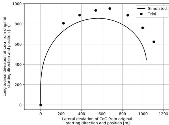
Figure 5: Comparison between results of simulation and trial of a 35° turning circle at a depth/draft ratio of 1.5 of the Esso Osaka at an approach speed of 7 knots.
