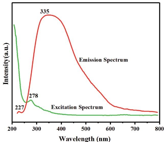
Fig. 4 Optical emission and excitation spectra of BNNTs.
