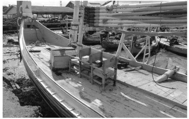
Fig. 3. The low bulwark and hatchway on Slerek fishing boat, Muncar
