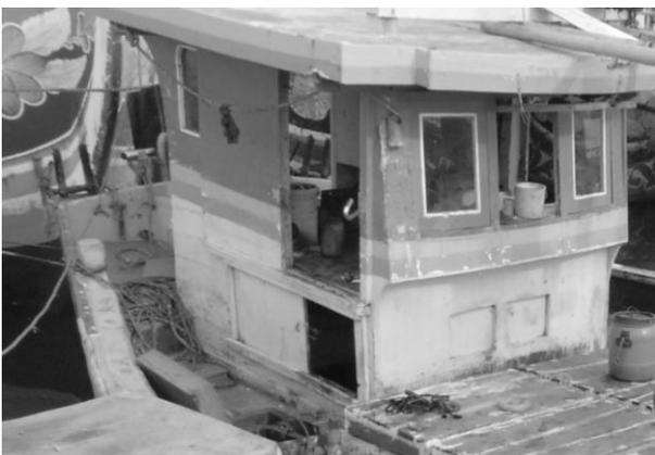
Fig. 2. The access to engine room below the sleeping space for crew
