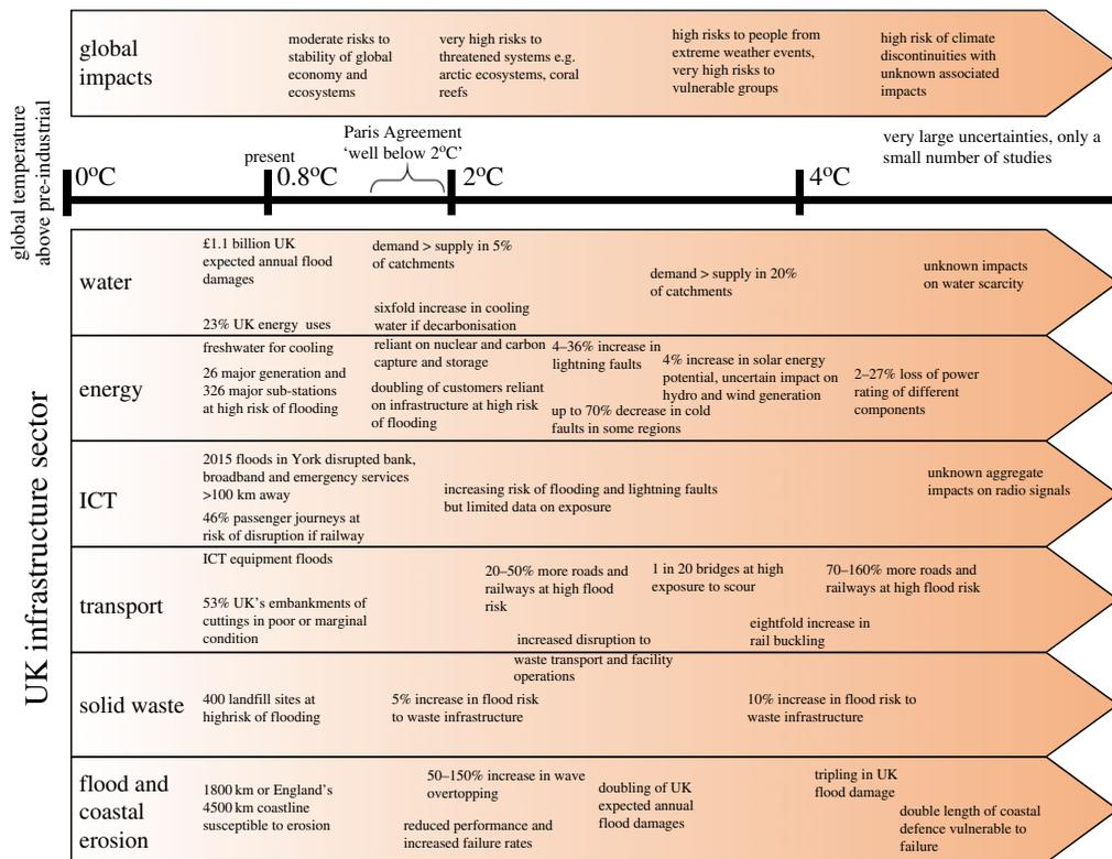
**Figure 4.** Relationship between global temperature change relative to pre-industrial era, and some of the key climate change risks to UK infrastructure. A high risk of flooding has a likelihood of flooding more frequently than 1 in 75 years ( $AEP \geq 0.013$ ). The assessment of global change risks is taken from [12]. (Online version in colour.)
