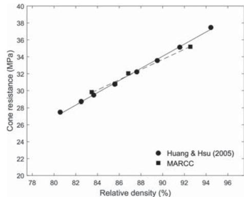
Figure 6. Comparison between CPT results obtained in Huang & Hsu's (2005) chamber and MARCC under BC5.
