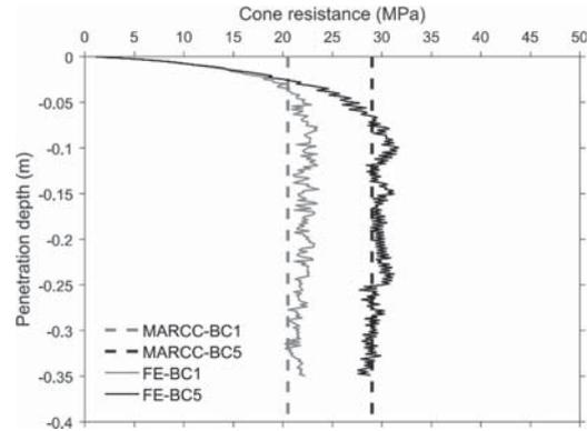
Figure 9. Numerical and experimental results for the uncalibrated CPTs in CC under BC1 and BC5. The straight-lines represent the average values of the steady state part of the experimental CPT curves.
