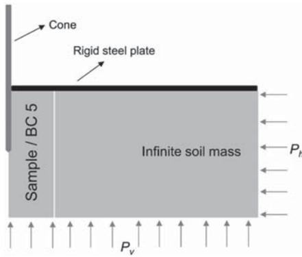
Figure 3. Axisymmetric schematic drawing of an ideal BC5 in the CC.
