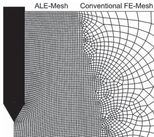
Figure 7. Deformed mesh around the cone in the FE model.
