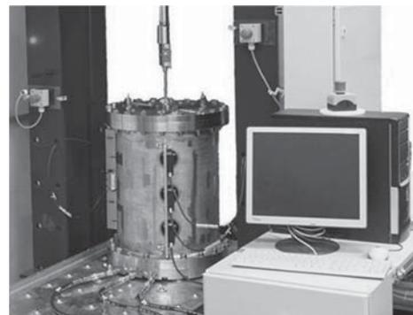
Figure 1. An overview of the calibration chamber facility MARCC at MARUM, University of Bremen.
