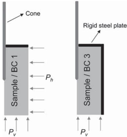
Figure 2. Axisymmetric schematic drawing of the BC1 and BC3 in the CC.
