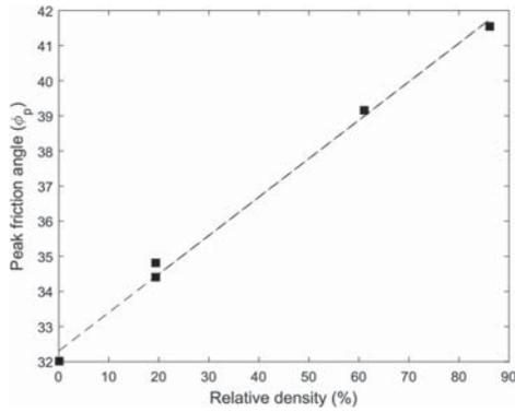
Figure 4. Peak friction angle as a function of relative density.
