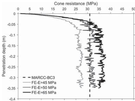
Figure 8. Three trial numerical CPT curves for CC test under BC3 with soil parameters presented in Table 1 and different Young's moduli, the straight-line represents the average value of the steady state part of the experimental CPT curve.
