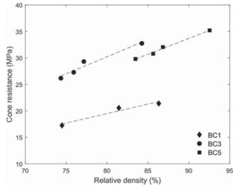
Figure 5. CPT results in Cuxhaven sand obtained in MARCC with different boundary conditions.
