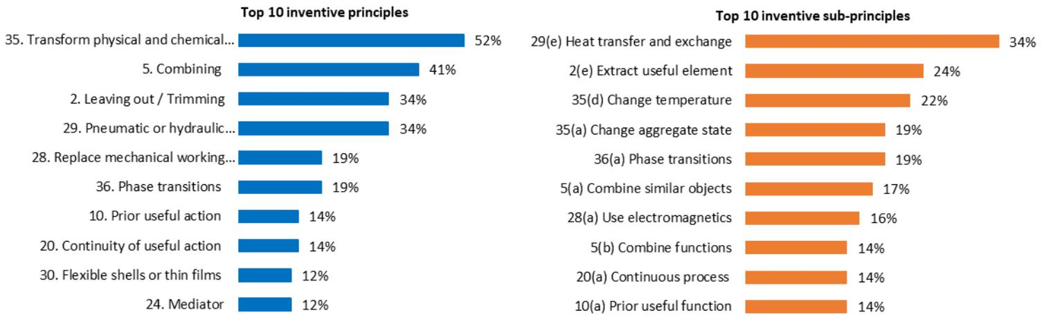
**Fig. 6.** Top 10 TRIZ inventive principles and sub-principles most frequently encountered in the 58 analyzed thermal operations and methods, presented in Table 7
