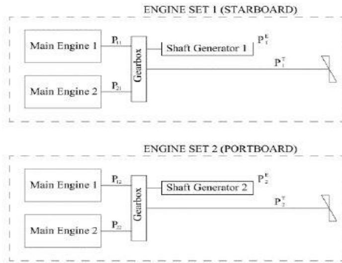
Figure 2: Engine room layout
