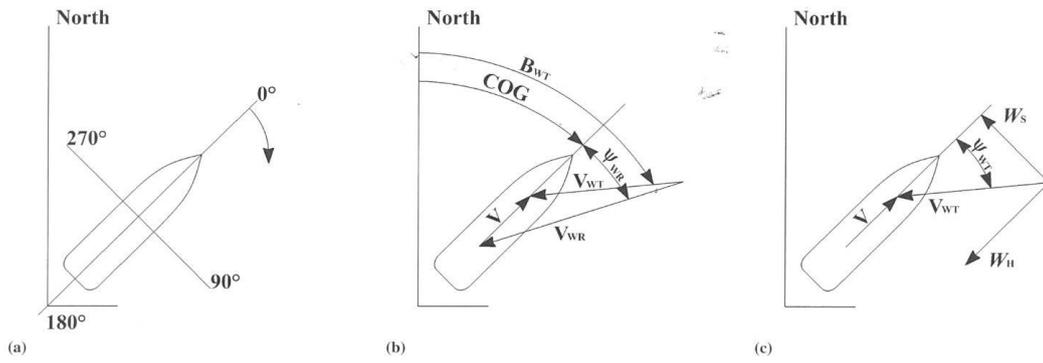
Figure 1: wind components
