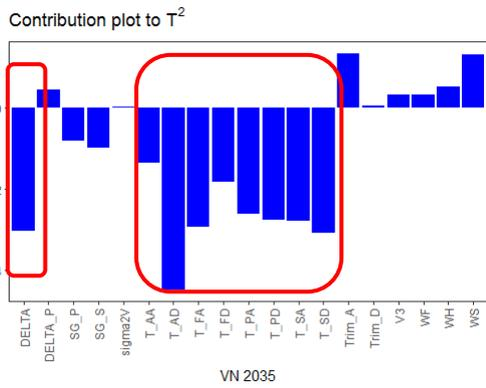
Figure 9: Contribution of the variables to the Hotelling  $T^2$  statistic, for the voyage 2035 of Ship 1.
