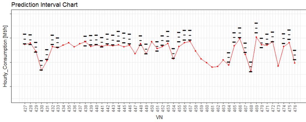
Figure 13: Prediction error control chart for voyages 427—476 of Ship 2, which follow an energy efficiency operation.
