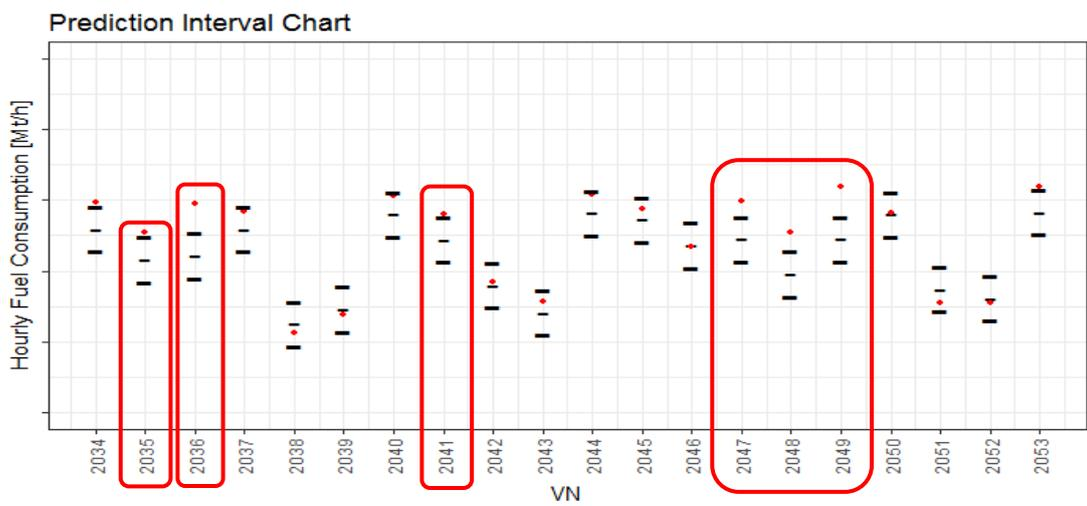
Figure 8: Prediction error control chart for voyages 2034–2053 of Ship 1.
