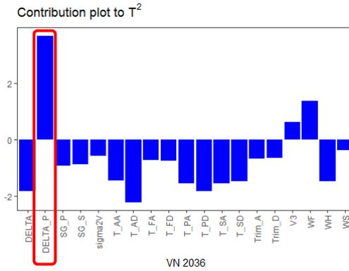
Figure 11: Contribution of the variables to the Hotelling  $T^2$  statistic, for the voyage 2036 of Ship 1.
