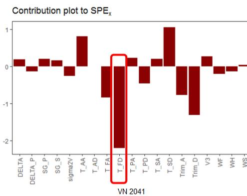
Figure 12: Contribution of the variables to the  $SPE_x$  statistic, for the voyage 2041 of Ship 1.
