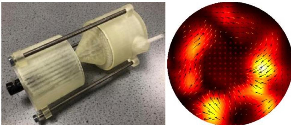
Figure 1: (L) 3D-printed miniature Torbed, (R) preliminary velocity field obtained via experimental particle image velocimetry
