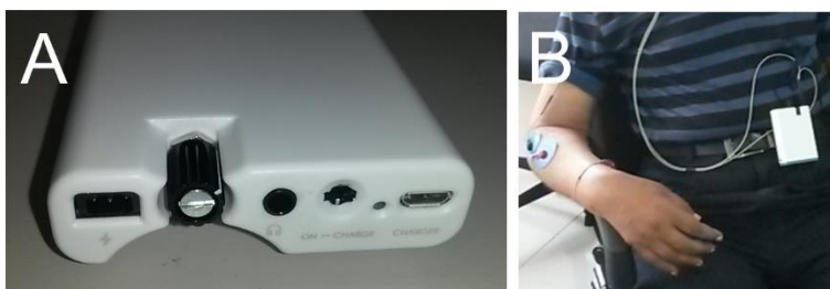
Figure 1. The experimental device. A, photograph of the device, showing (from left to right): connector for stimulating electrodes; knob for adjusting stimulus intensity; audio output to earpiece; switch to select between 'on' and 'charge'; LED to indicate when battery is fully charged; microUSB connector for charger. B, device in use by a stroke patient in Kolkata as part of the trial to improve hand function.
