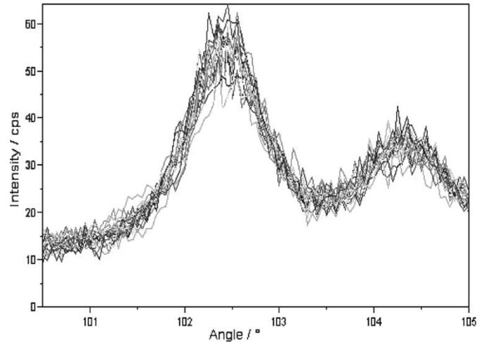
Fig. 2. Representative diffraction peaks of the analyzed samples.
