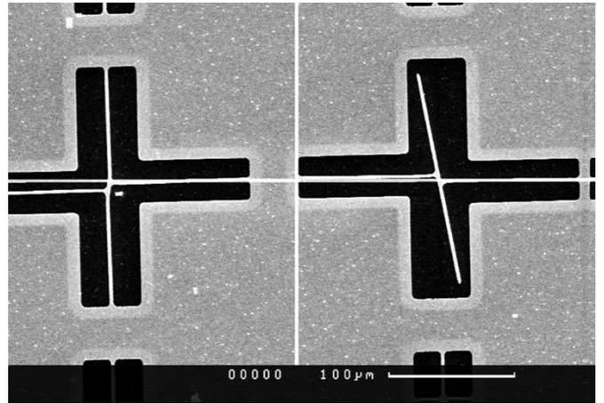
Fig. 7. Scanning electron micrograph of two adjacent sensors on a polyimide dielectric, showing the origin of the enhanced rotation.
