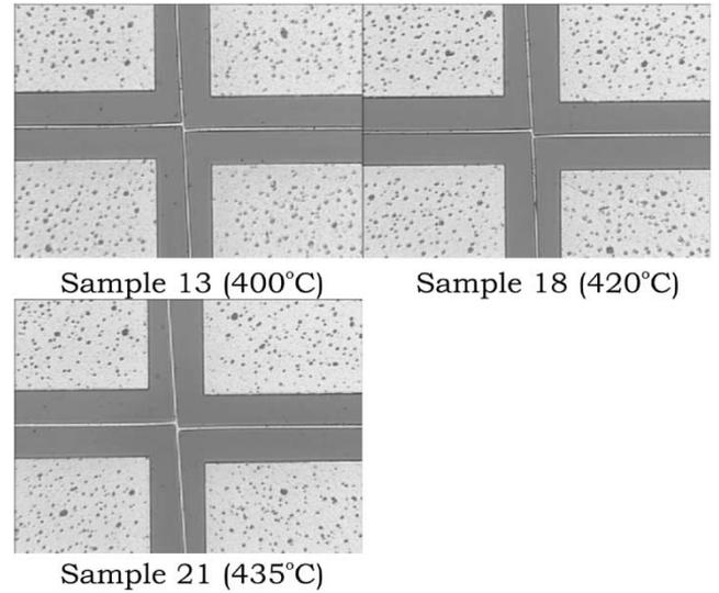
Fig. 4. Reflected light micrographs for sensor structures with 1-μm feature width fabricated on SiO<sub>2</sub> intermetal dielectric after different sinter hold temperatures.
