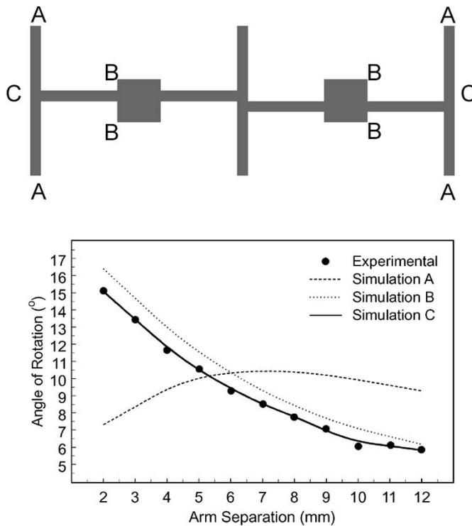
Fig. 8. Influence of the anchor points on the angle of rotation and experimental data for a sensor of identical dimensions.
