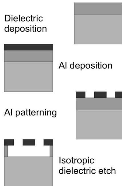
Fig. 3. Cross-sectional process flow.
