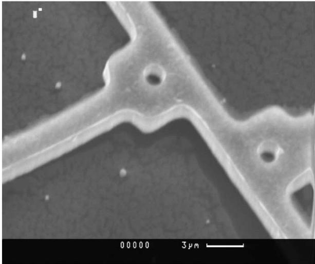
Fig. 5. Scanning electron micrograph of the hinge region of a sensor designed for reducing plastic deformation [11], showing feature rounding from the photolithographic process.
