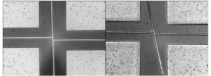
Fig. 6. Reflected light micrographs for sensor structures with  $1\text{-}\mu\text{m}$  feature width. (left)  $\text{SiO}_2$  dielectric, (right) polyimide dielectric.
