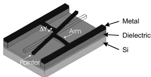
Fig. 1. Three-dimensional (3-D) isometric view of the sensor structure.
