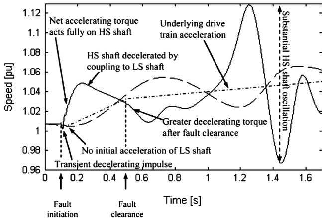
Fig. 18. Speed-time response of wind farm drive train.
