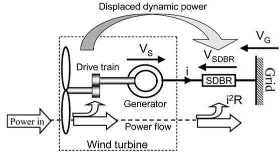
Fig. 2. Conceptual benefit of SBDR under fault conditions.
