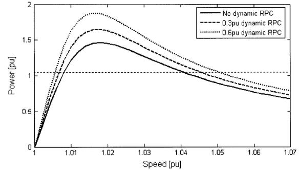
Fig. 9. Effect of dynamic RPC on steady-state characteristics.
