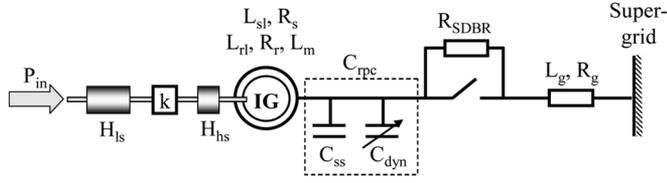
Fig. 5. Reduced schematic of representative wind farm.
