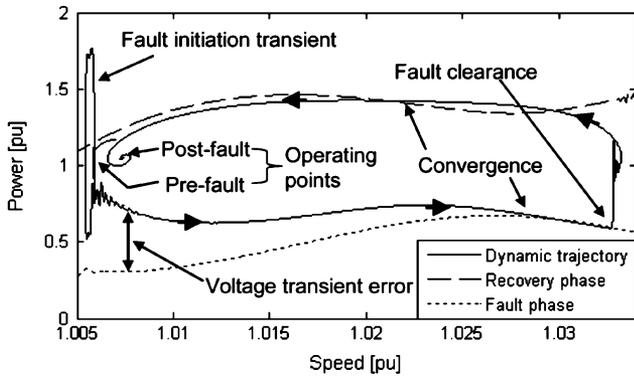
Fig. 17. Correlation of dynamic simulation with quasi-steady-state.
