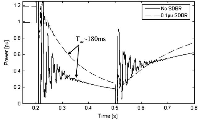
Fig. 14. Transition of mechanical power during fault N.
