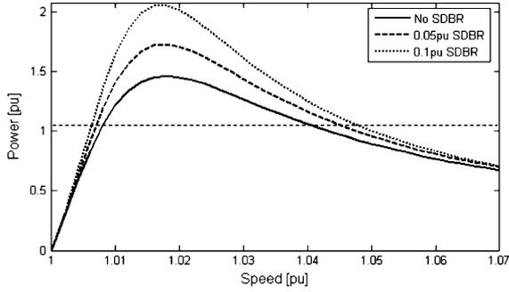
Fig. 11. Effect of dynamic SDBR on steady-state characteristics.
