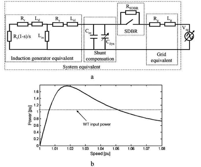
Fig. 7. Equivalent circuit and power curve for representative wind farm. (a) Equivalent circuit. (b) Decelerating power versus speed characteristic (rated grid voltage).
