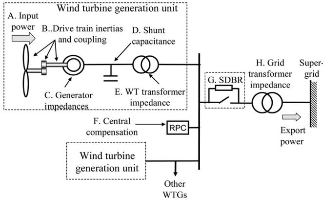
Fig. 4. Typical large wind farm single line diagram.
