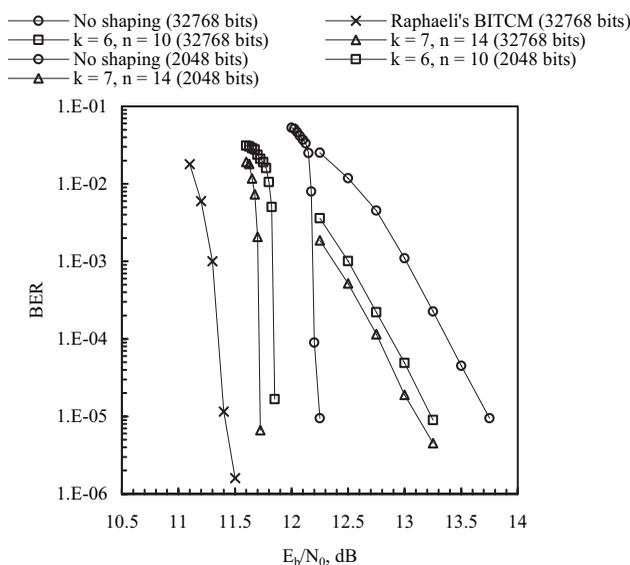
Fig. 4. Performance comparison over Gaussian channel between several 3-bit/dim 16-PAM BITCMs for 32768-bit and 2048-bit interleaving. The turbo codes based on 32768-bit and 2048-bit interleaving use 18 and 10 decoding iterations, respectively. The BITCMs with shaping code employ either the ( $R_c = 5/6, k = 6, n = 10$ ) configuration or the ( $R_c = 6/7, k = 7, n = 14$ ) configuration, while the BITCMs without shaping use a rate-3/4 turbo code.
