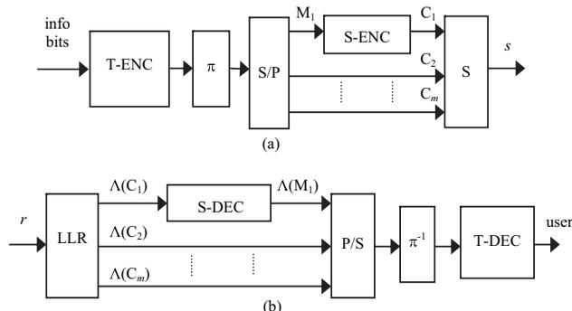
Fig. 1. Structure of the proposed BITCM scheme: (a) transmitter, (b) receiver.
