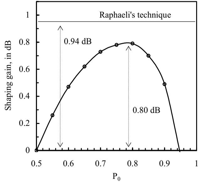
Fig. 3. Variation of the achievable shaping gain as a function of  $P_0$  for the proposed system, when  $C = 3$  bits/dim and  $m = 4$  (16-PAM).
