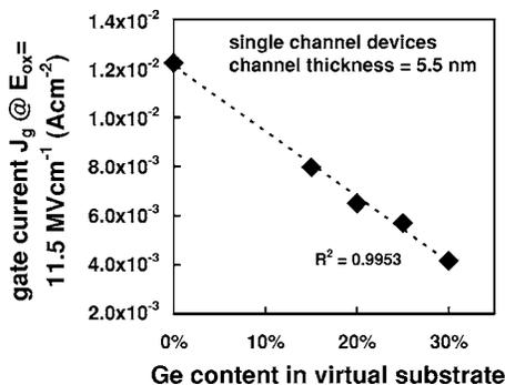
FIG. 3. Gate leakage ( $J_g$ ) vs virtual substrate Ge content at a gate oxide electric field ( $E_{ox}$ ) of  $11.5 \text{ MV cm}^{-1}$  (FN dominated).
