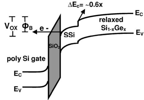
FIG. 4. Strained Si band structure when a positive gate voltage is applied.
