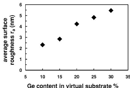
FIG. 8. Surface roughness vs virtual substrate Ge content measured by AFM.
