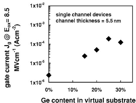
FIG. 5. Gate leakage ( $J_g$ ) vs virtual substrate Ge content at a gate oxide electric field ( $E_{ox}$ ) of  $8.5 \text{ MV cm}^{-1}$  (PF dominated regime).
