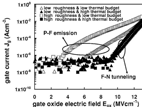
FIG. 9. Gate leakage ( $J_g$ ) characteristics for dual channel strained Si *n*-MOSFETs.
