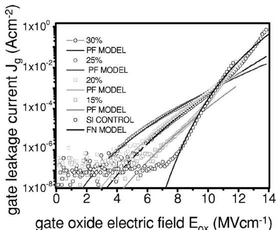
FIG. 6. Measured and modeled gate leakage characteristics for strained Si single channel *n*-MOSFETs fabricated on relaxed SiGe virtual substrates with Ge contents ranging from 0% to 30%. MOSFETs have 5.5 nm strained Si channel thicknesses.
