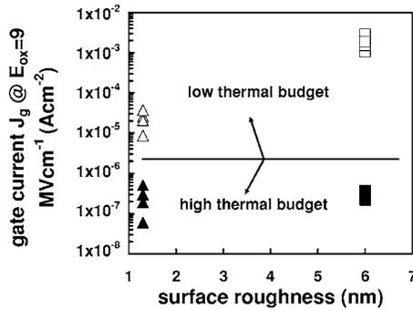
FIG. 10. Impact of thermal budget and epitaxial surface roughness on gate leakage ( $J_g$ ) at an oxide electric field ( $E_{ox}$ ) of  $9 \text{ MV cm}^{-1}$ .
