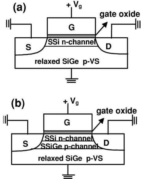
FIG. 1. MOSFET architectures: (a) single channel devices and (b) dual channel devices.
