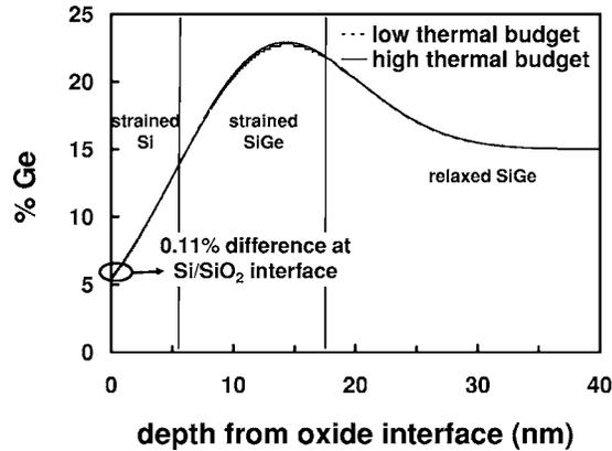
FIG. 2. MEDICI simulated Ge profiles indicating as-grown layer specification and profiles after low and high thermal budget MOSFET processes. The low thermal budget corresponds to unsalicyded devices and the high thermal budget corresponds to salicyded devices.
