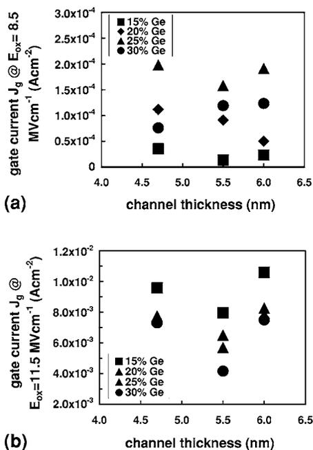
FIG. 7. Impact of strained Si channel thickness on (a) PF emission and (b) FN leakage in single channel *n*-MOSFETs.
