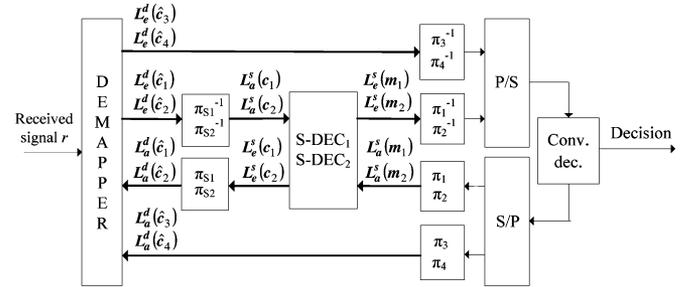
Fig. 3. Structure of the 16-QAM BICM-ID receiver.
