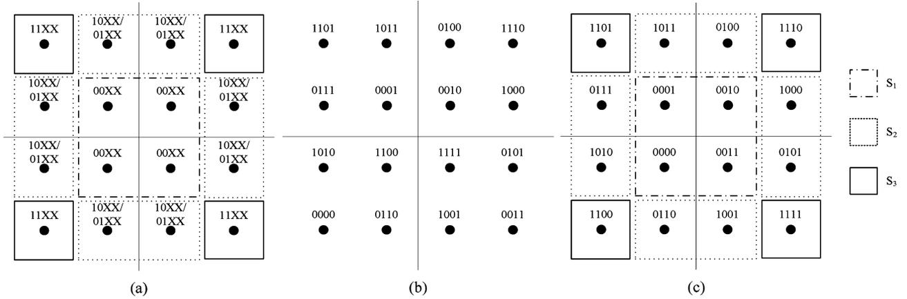
Fig. 2. Different mappings for 16-QAM. (a) 16-QAM mapping required for the BICM-ID system with constellation shaping. (b) Schreckenbach's mapping. (c) Modified Schreckenbach's mapping.
