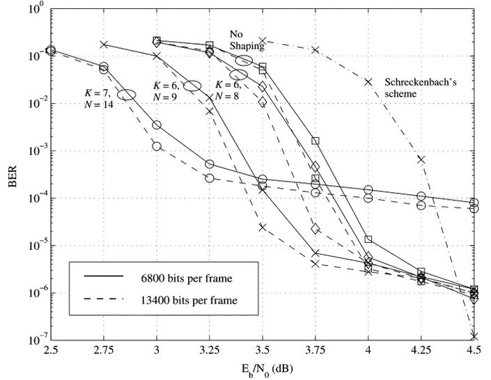
Fig. 4. Performance comparison over Gaussian channel between several 2-b/s/Hz 16-QAM BICM-ID scheme using convolutional coding with 10 iterations and frame sizes  $N_b = 6800$  and 13400 information bits per frame. Performance of equivalent BICM-ID system without shaping is also shown.
