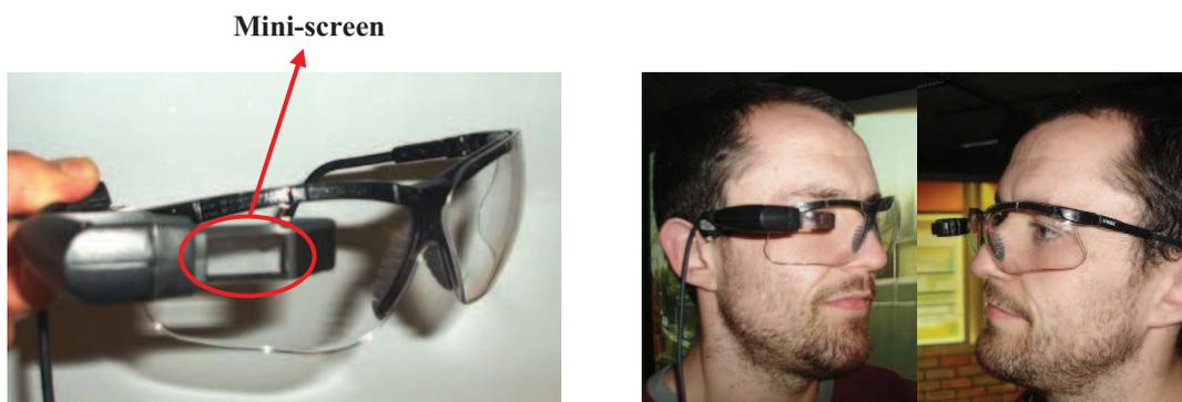
**Figure 4: The Wearable Display**
