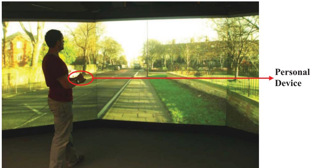
**Figure 2: A subject stands in the middle of the cave-based immersive display formed by three screens**
